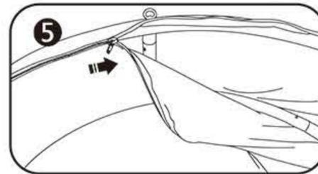
If can't snap when dismantle the frame,Pls push the tube forwardly,then push again.
